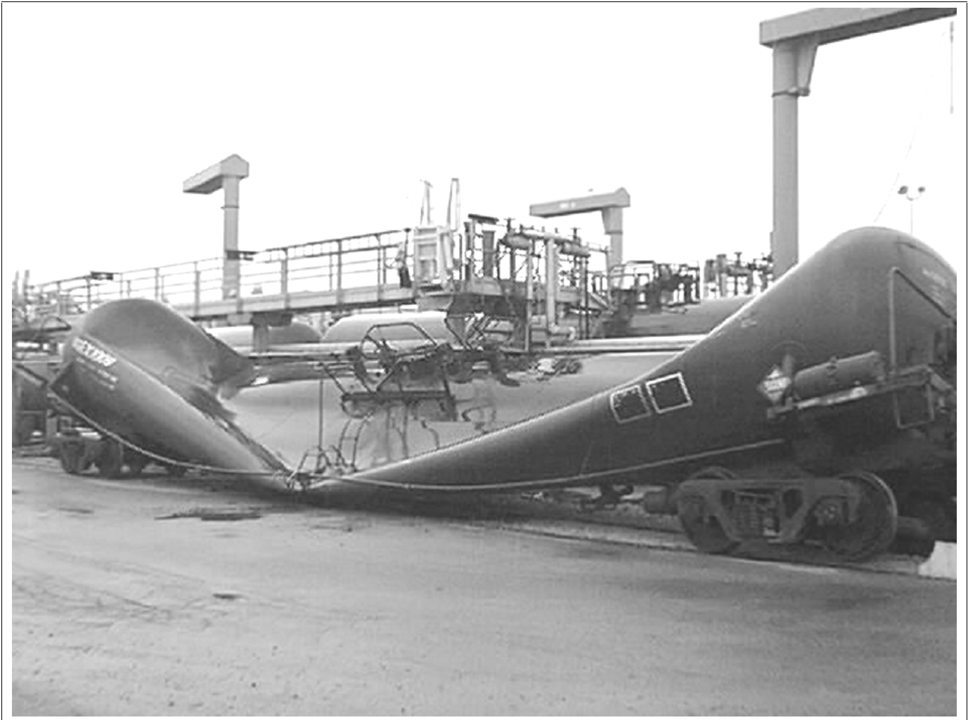
Figure 29 Natural Vacuum Principle Demonstrated
