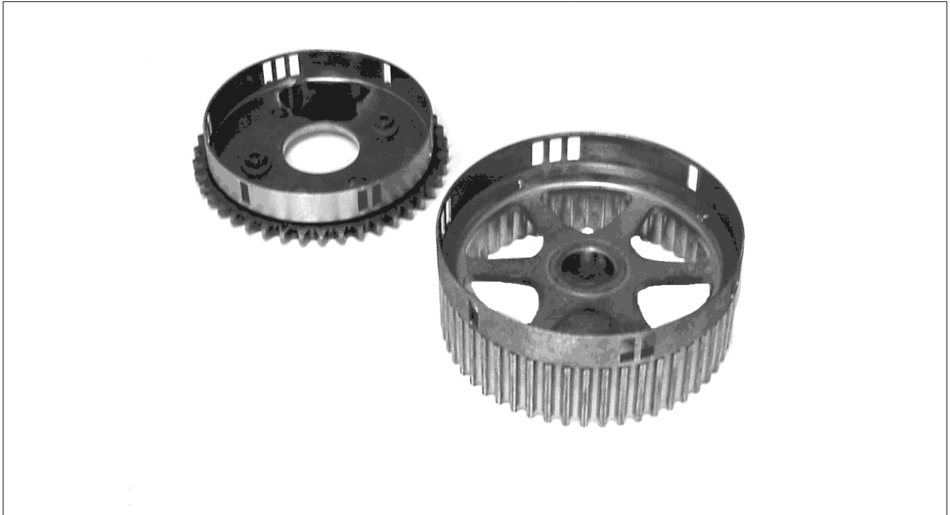
Figure 12 Typical 6 Cylinder CMP Triggers (2.7L / 3.5L shown)
